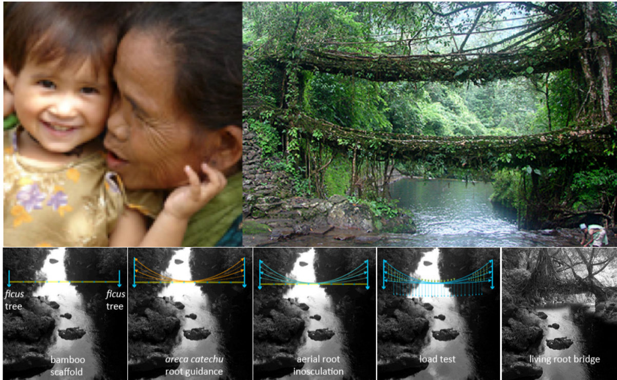
Fig 2. Khasi tribes and living root bridge growth process
